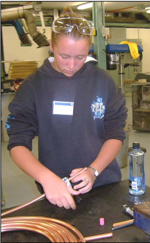
Lucy Suthern cutting copper pipe in the Refrigeration and Air Conditioning workshop
